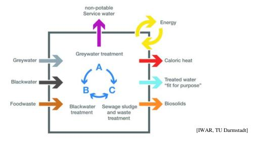
Figure 1 Mass flow in the semi-centralised Resource Recovery Center
